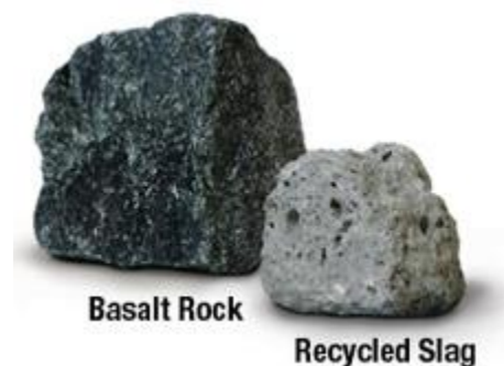
Figure 1: Basalt Rock and Recycled Slag
